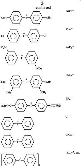
In the practice of the invention, the iodonium bisul-45 fate salt is initially formed by agitating a mixture of aromatic compound, potassium iodate, methylene chloride, sulfuric acid and acetic anhydride. Suitable aromatic compounds include, for example, benzene, toluene, o-xylene, m-xylene, p-xylene, chlorobenzene, bromobenzene, alkylbenzene, nitrobenzene, N-phenyl- 50 maleimide.
