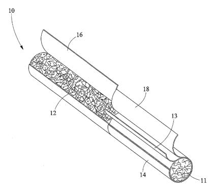
(57) Abstract: A method of flavoring a filter plug wrap (13) of a smoking article (10), such as a cigarette, is disclosed. Furthermore, a method of incorporating flavoring into the plug wrap (13) and using the plug wrap (13) to wrap the filter (14) of the smoking article (10) is disclosed. A smoking article (10) and a filter (14) having a flavored filter plug wrap (13) are also disclosed.
