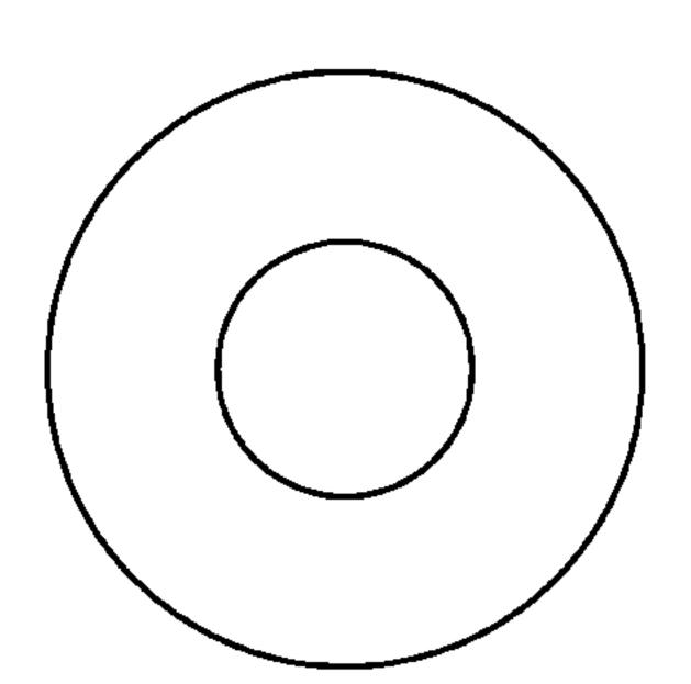
(57) Abstract: A bushing-like part made from a fluoropolymer and circumferentially oriented continuous high tensile modulus fibers is useful as a part for pumps and compressors and other similar types of apparatus. These parts may be useful at high temperatures and/or very corrosive environments, often lengthen the time between required maintenance checks, and usually perform better than metal bushings under nonstandard operating conditions.
