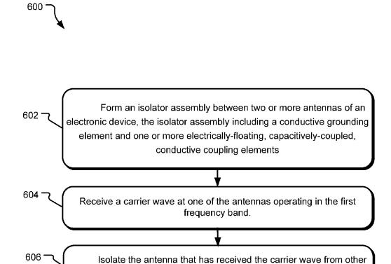
antennas positioned on an opposite side of the isolator assembly.
