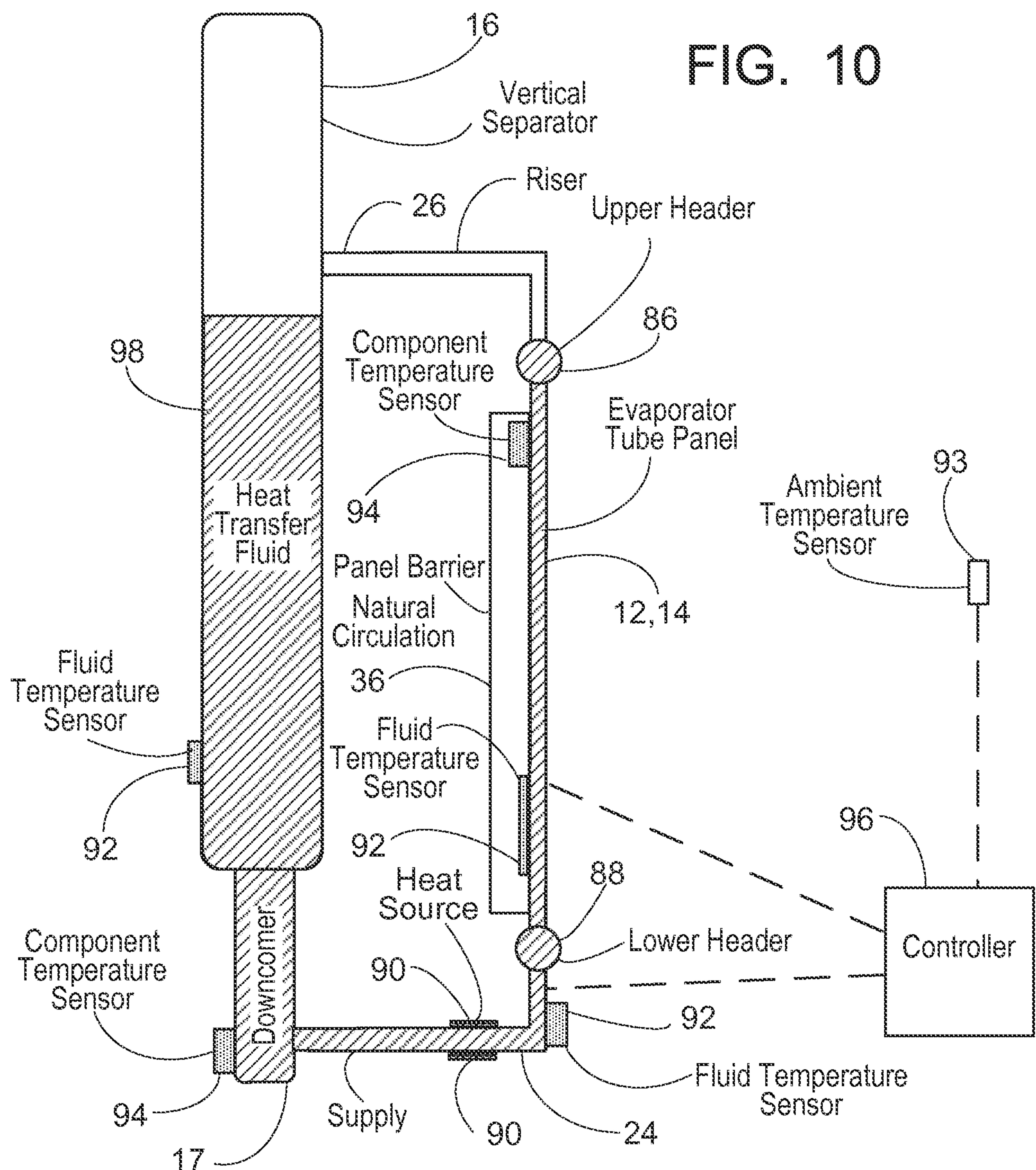
Freeze Protection Via Heat Source Located On
