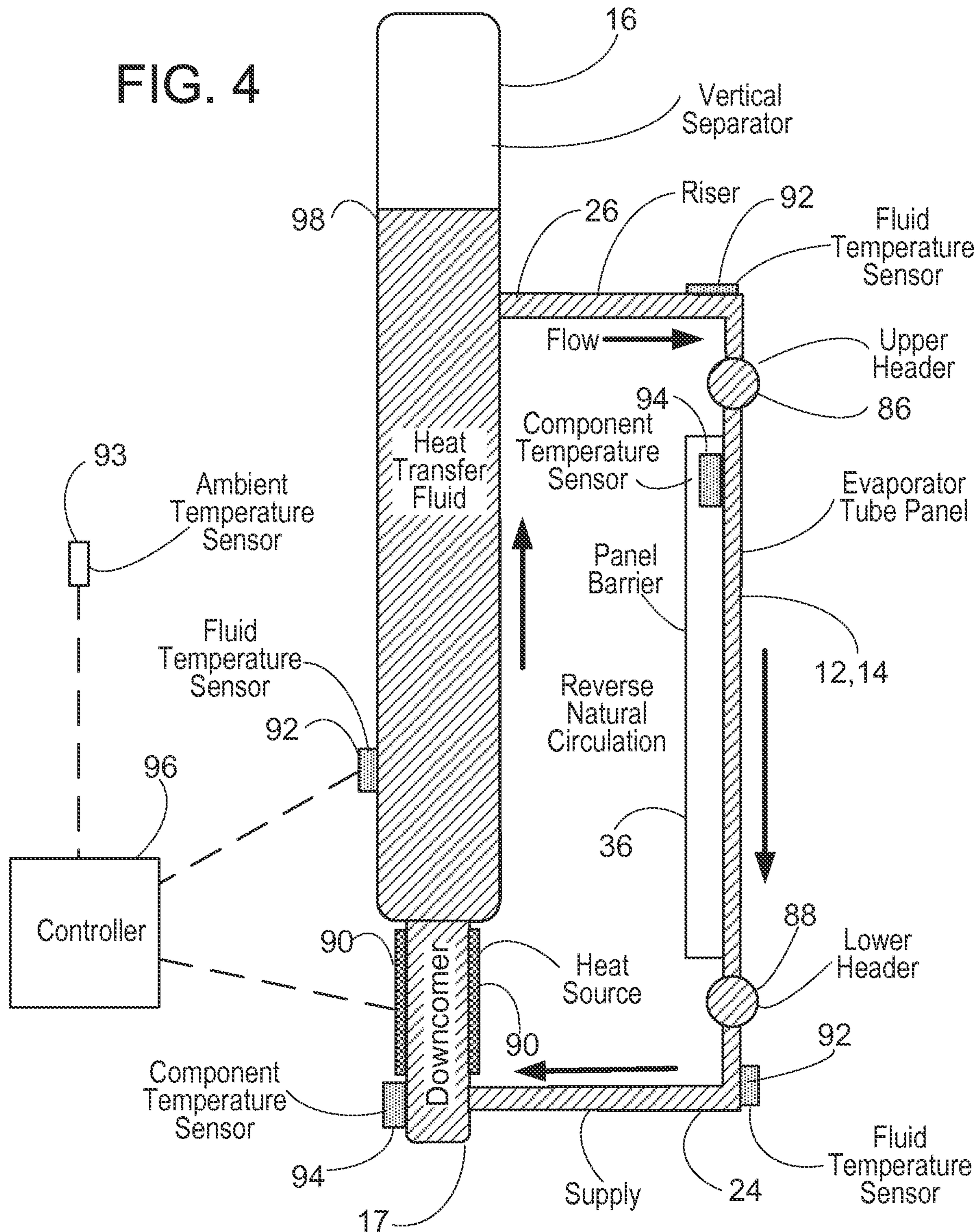
Freeze Protection Via Heat Source Located On
