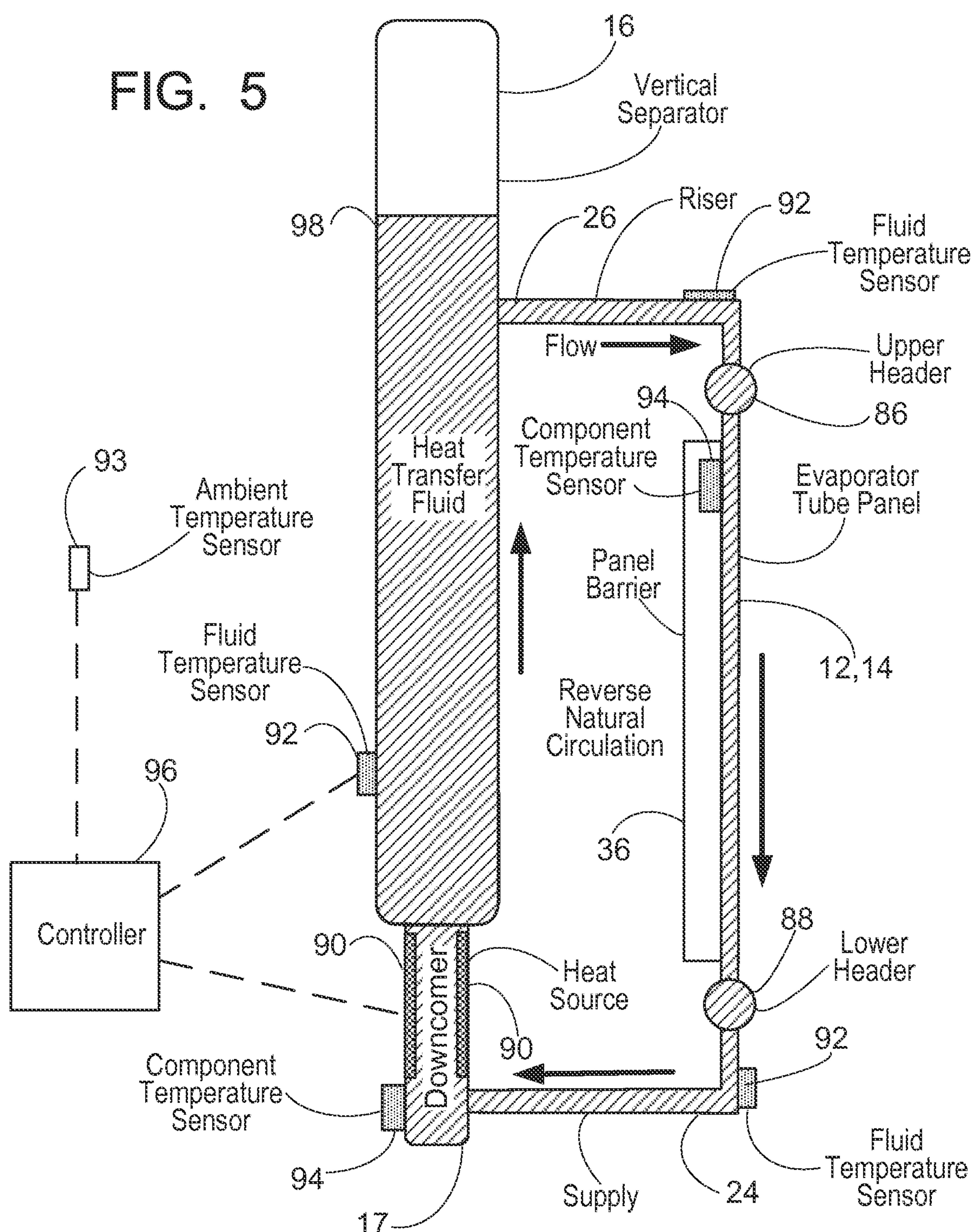
Freeze Protection Via Heat Source Located
