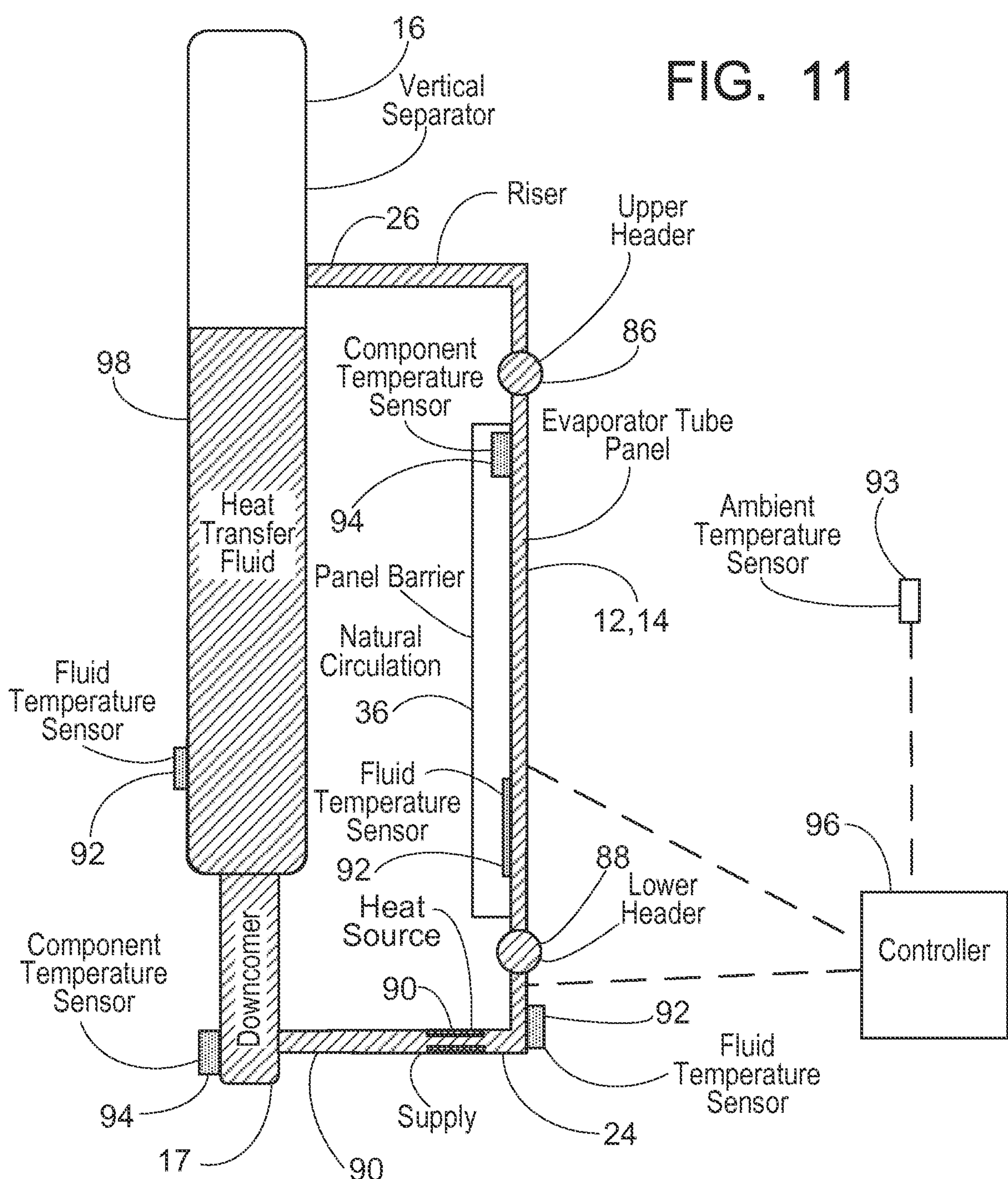
Freeze Protection Via Heat Source Located On
