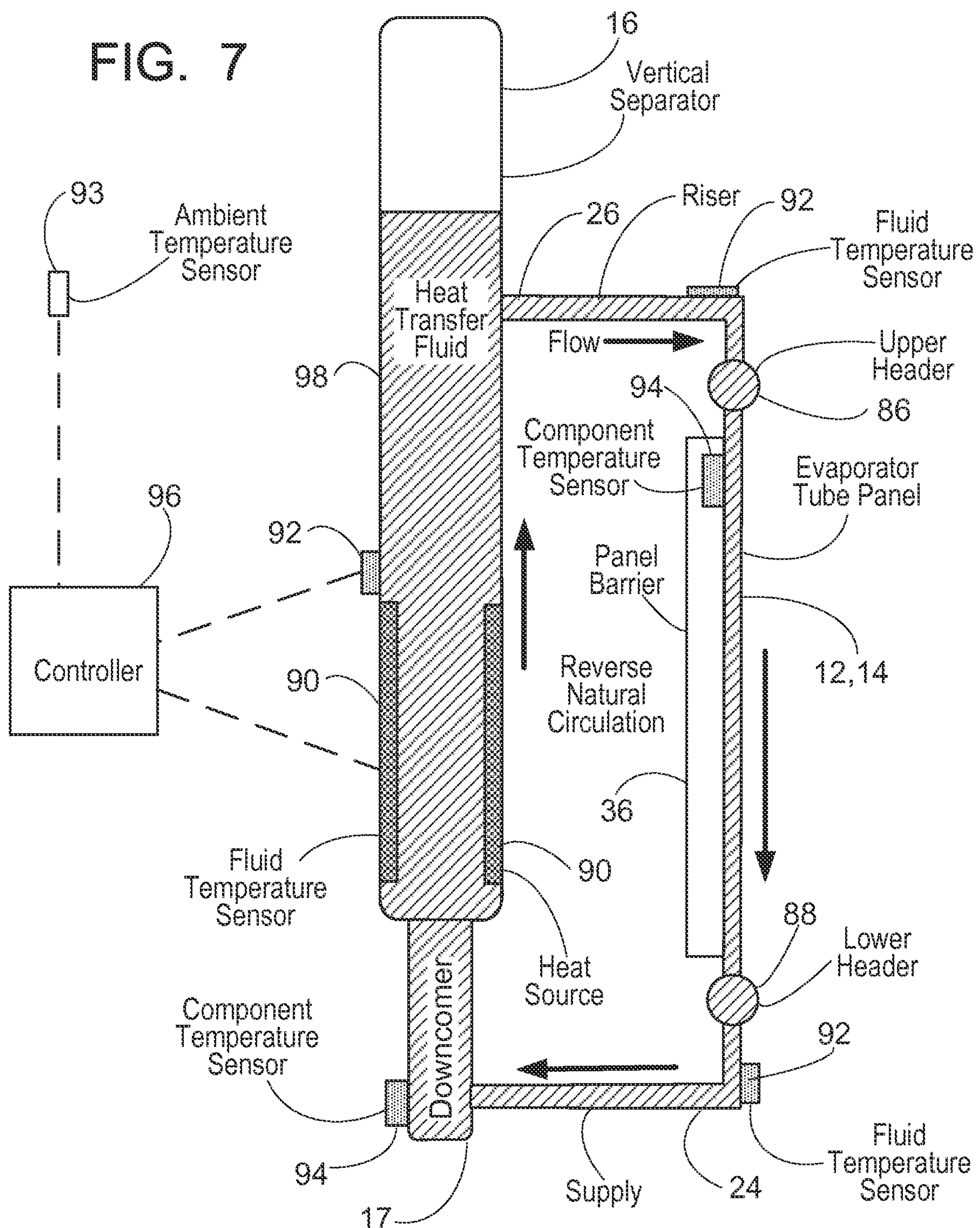
Freeze Protection Via Heat Source Located On
