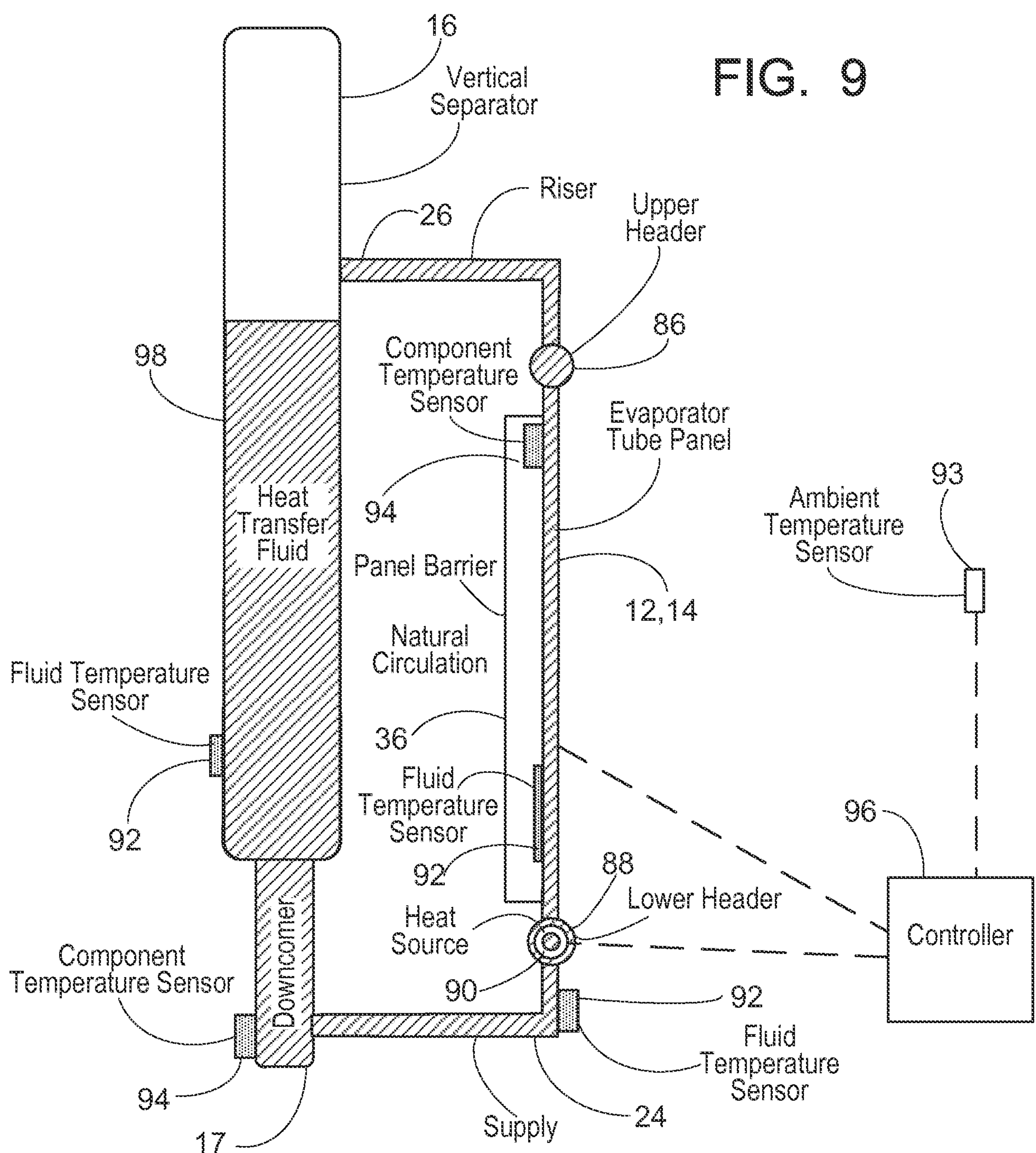
Freeze Protection Via Heat Source Located
