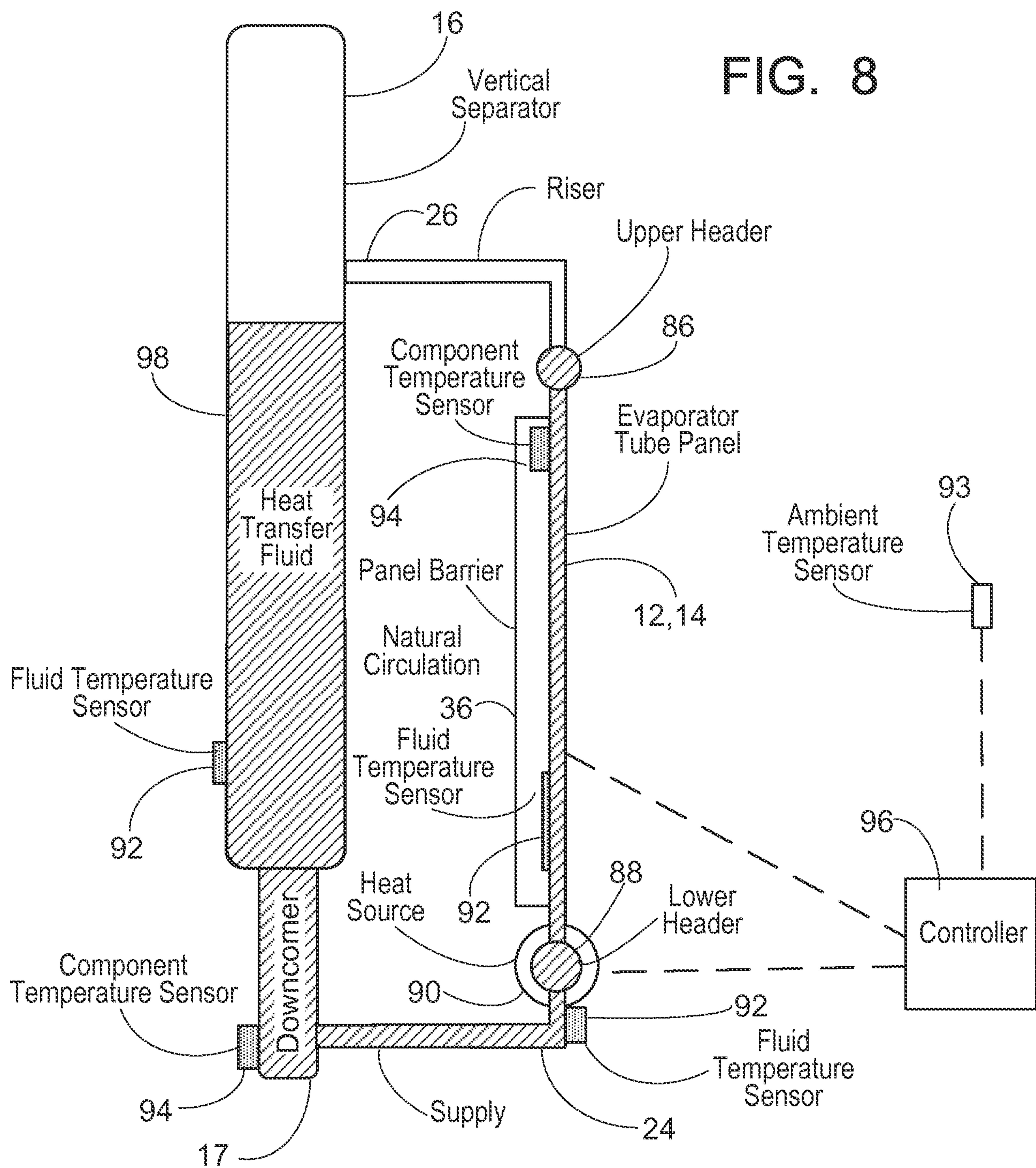
Freeze Protection Via Heat Source Located On
