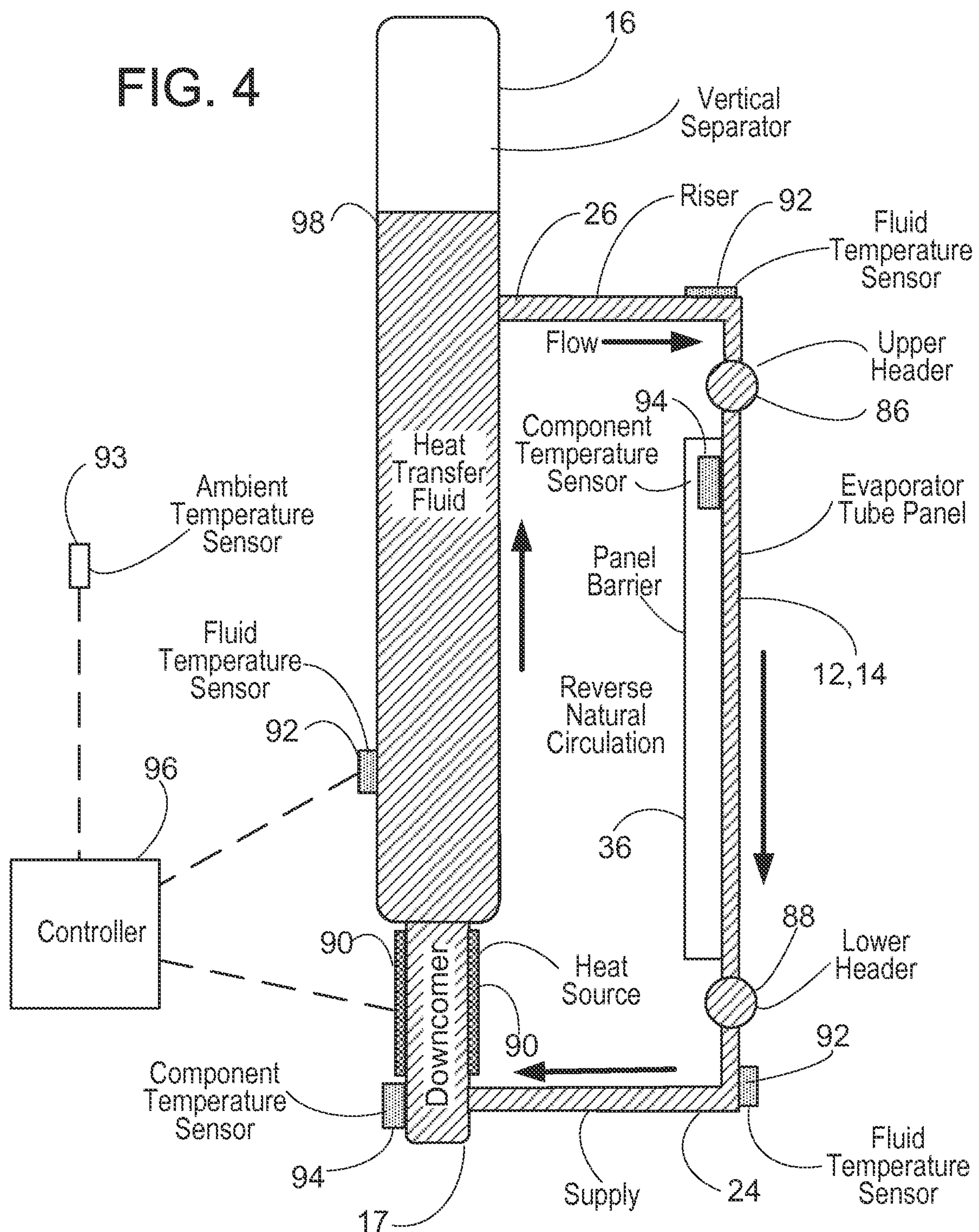
Freeze Protection Via Heat Source Located On
