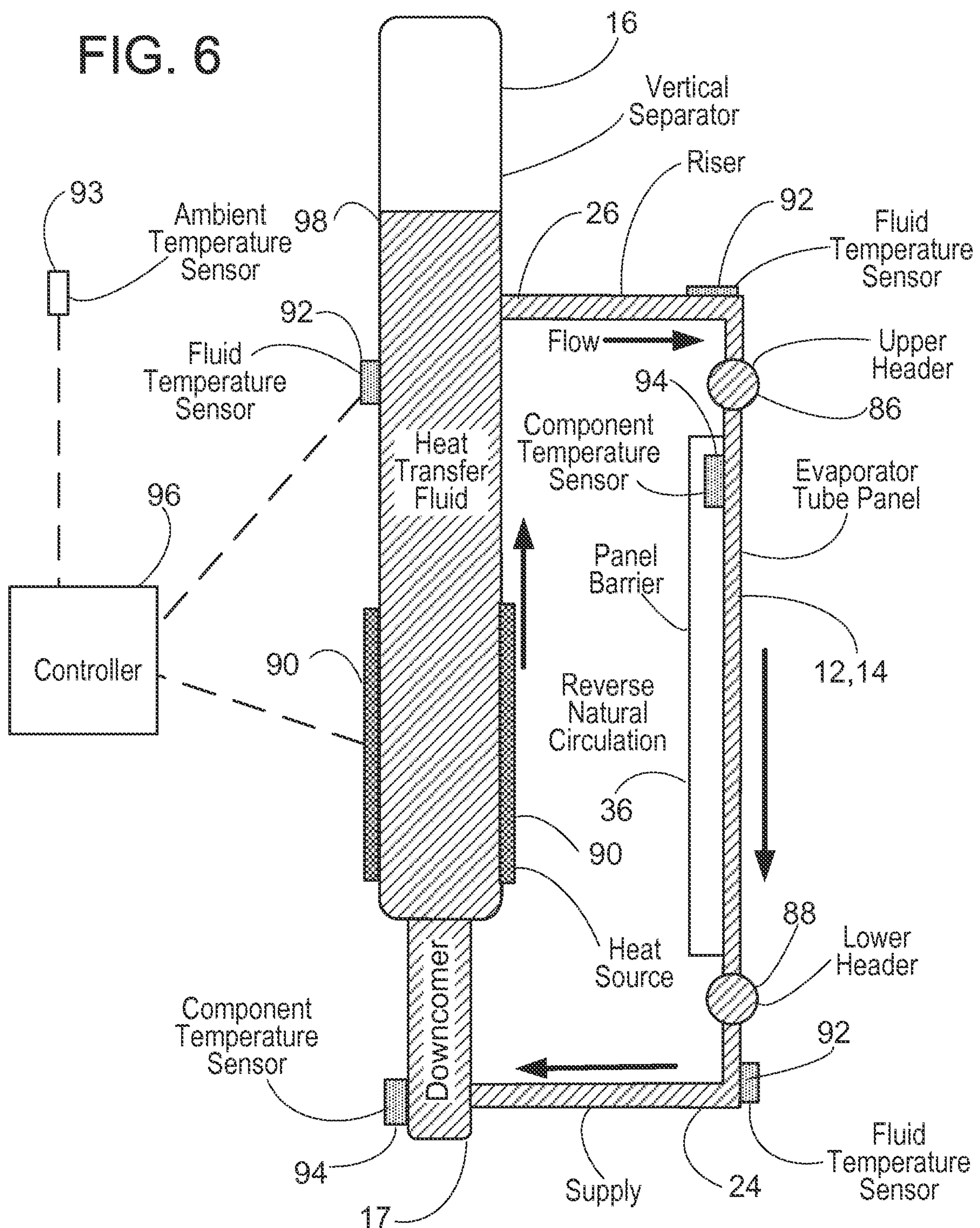
Freeze Protection Via Heat Source Located On
