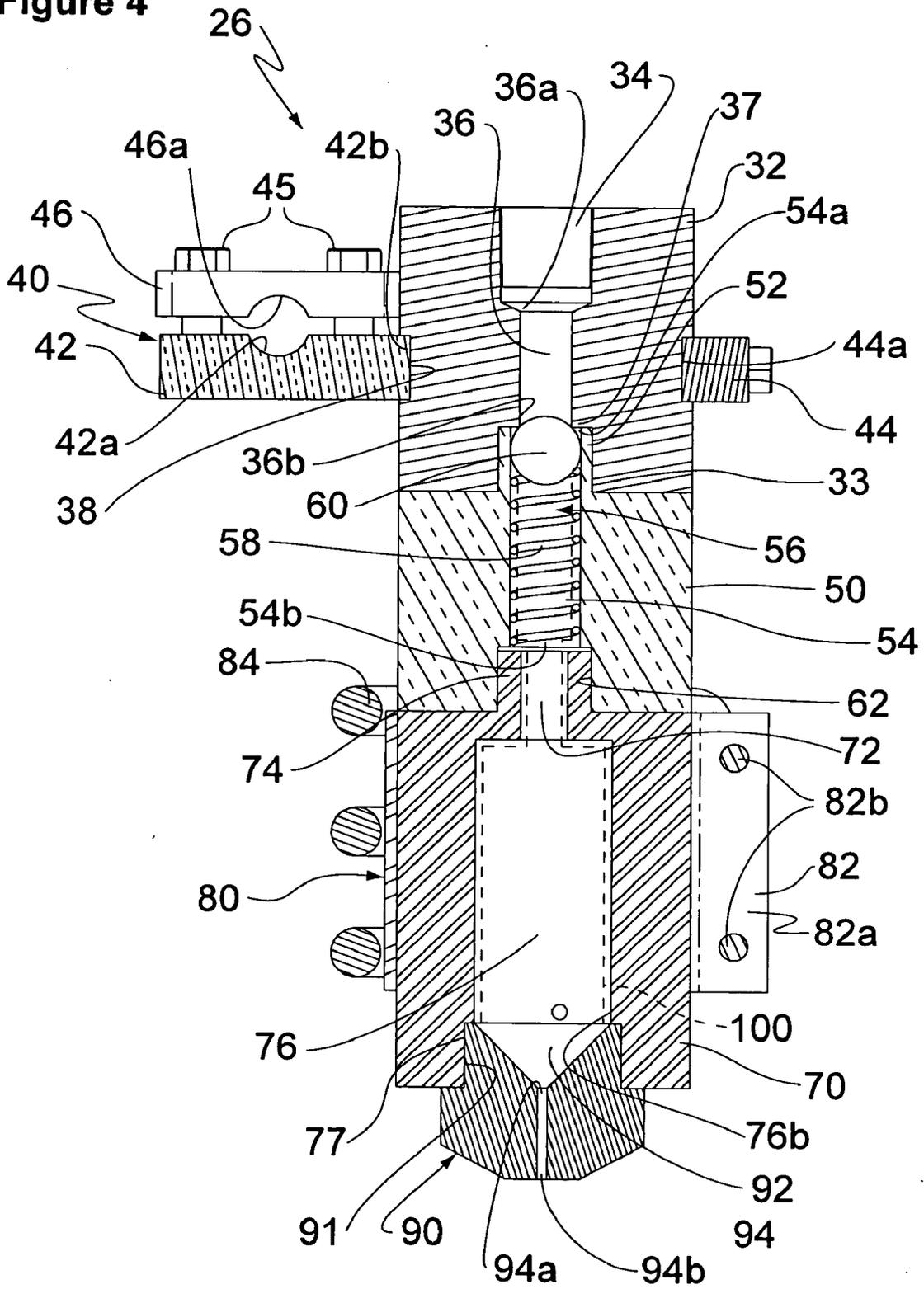
**SUBLIMATION PEN FOR USE IN A DYE SUBLIMATION PRINTING SYSTEM, AND METHOD OF USE OF THE DYE SUBLIMATION PRINTING SYSTEM**
