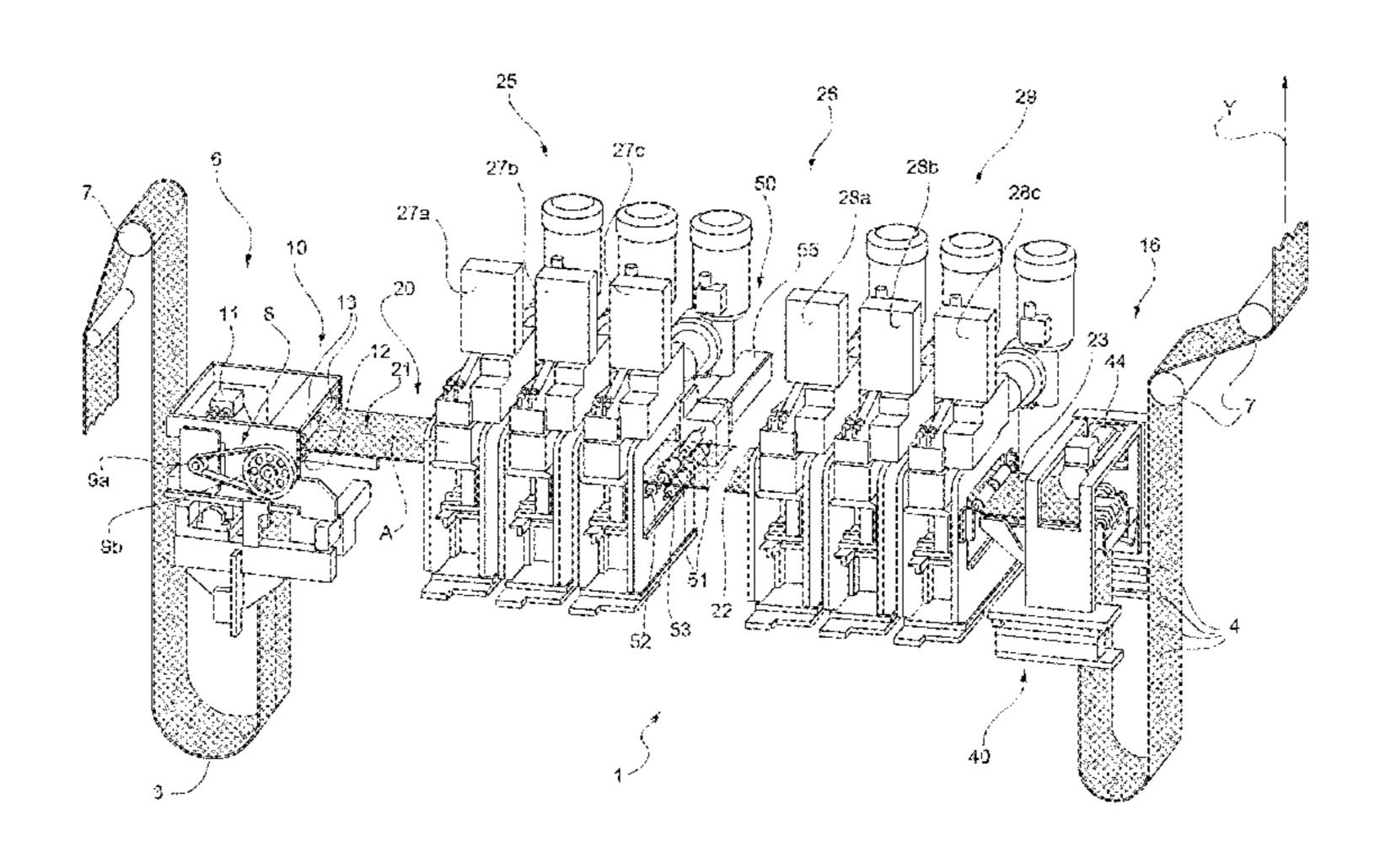
second distance along direction; feeding group comprises: advancing device controllable to arrest web in a position, at which second area is spaced an intentional offset from second desired position; and an actuator controllable for moving second area towards second desired position to recover offset; absolute value of difference between first and distances being equal to offset.
