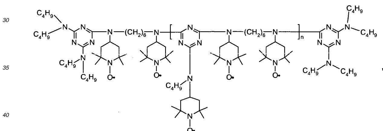
45 which is the oxidation product of Chimassorb 2020 (RTM). Chimassorb 2020 is described in EP 782 994, n is a mixture of numbers between 1 and 10.  $M_w$  (by GPC) is approximately 3000 and  $M_w/M_n$  is typically 1.2.
