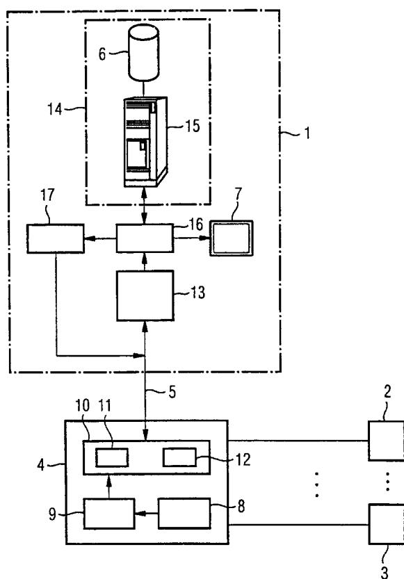
(57) Abstract: The invention relates to a method for signaling and processing incoming calls for a call center. The invention further relates to a corresponding exchange and a corresponding call center. According to the invention, incoming calls for the call center and the subscriber numbers of the callers are signaled to the call center by the exchange via an internet protocol link between the exchange and the call center.
