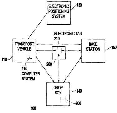
(57) Abstract: An inventive system (100) for delivering a package (200) or plurality of packages, includes a transport vehicle (110) for transporting the package (200) to a destination (140), the transport vehicle (110) including a first transceiver and a computer system (115), and an electronic positioning system (130) for navigating the transport vehicle to the destination under a low-visibility condition
