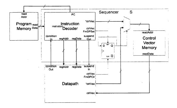
Figure 2: Sequencer for Functional Unit
