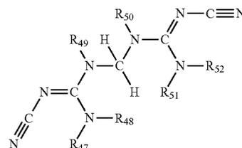
wherein R<sub>47</sub>, R<sub>48</sub>, R<sub>49</sub>, R<sub>50</sub>, R<sub>51</sub> and R<sub>52</sub> are one or more members independently selected from the group consisting of: H, and —CH<sub>2</sub>OH
