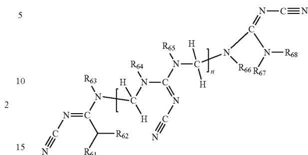
wherein  $R_{61}$ ,  $R_{62}$ ,  $R_{63}$ ,  $R_{64}$ ,  $R_{65}$ ,  $R_{66}$ ,  $R_{67}$  and  $R_{68}$  are one or more members independently selected from the group consisting of: H and  $-\text{CH}_2\text{OH}$  wherein x is 2-20.
