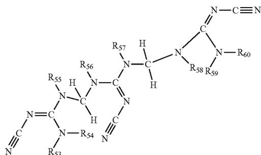
wherein R<sub>53</sub>, R<sub>54</sub>, R<sub>55</sub>, R<sub>56</sub>, R<sub>57</sub>, R<sub>58</sub>, R<sub>59</sub> and R<sub>60</sub> are one or more members independently selected from the group consisting of: H and —CH<sub>2</sub>OH
