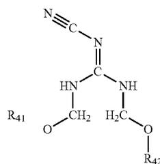
wherein  $R_{41}$  &  $R_{42}$ =H or  $\text{CH}_2\text{—OR}_{43}$
