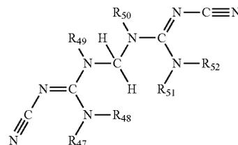
wherein  $R_{47}$ ,  $R_{48}$ ,  $R_{49}$ ,  $R_{50}$ ,  $R_{51}$  and  $R_{52}$  are one or more members independently selected from the group consisting of: H, and  $-\text{CH}_2\text{OH}$
