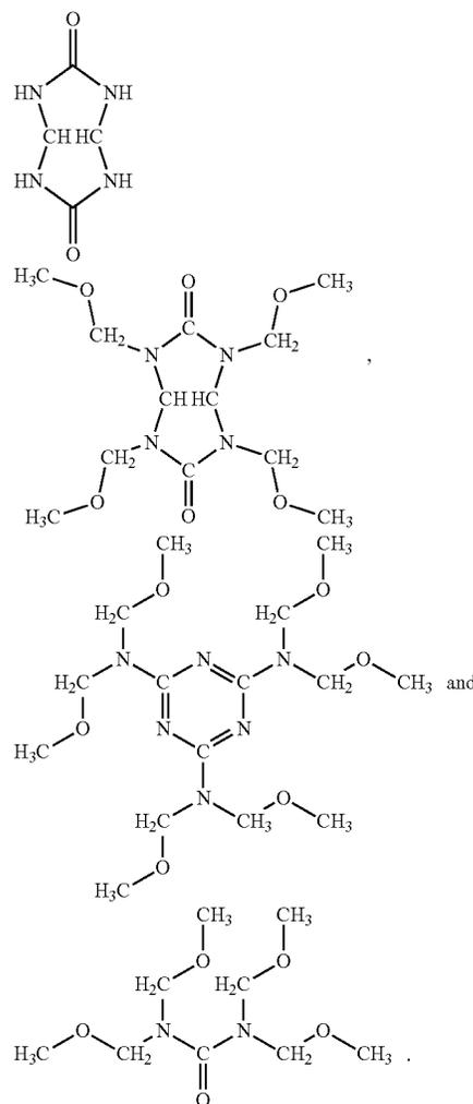
In an embodiment, the present invention relates to a composition of the biodegradable, hydrophobic polymers which comprises the reaction products of aldehyde(s) and nitrogen containing compounds dispersed in NOSDS wherein the one or more biodegradable hydrophobic polymers are present in an amount that is between about 5-65% of a total composition. In a variation, the crosslinking agent is present in an amount that is between about 0.1-10% of the total composition.
