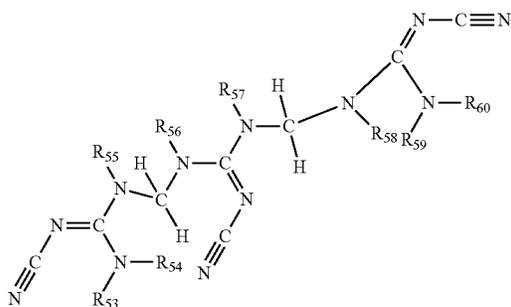
wherein  $R_{53}$ ,  $R_{54}$ ,  $R_{55}$ ,  $R_{56}$ ,  $R_{57}$ ,  $R_{58}$ ,  $R_{59}$  and  $R_{60}$  are one or more members independently selected from the group consisting of: H and  $-\text{CH}_2\text{OH}$ , wherein said structures are made by using non-aqueous conditions, and wherein the structures comprise more than 10% by weight of the nitrification inhibitor composition.
