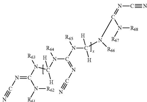
wherein  $R_{61}$ ,  $R_{62}$ ,  $R_{63}$ ,  $R_{64}$ ,  $R_{65}$ ,  $R_{66}$ ,  $R_{67}$  and  $R_{68}$  are one or more members independently selected from the group consisting of: H and  $-\text{CH}_2\text{OH}$  and wherein  $x=2-20$
