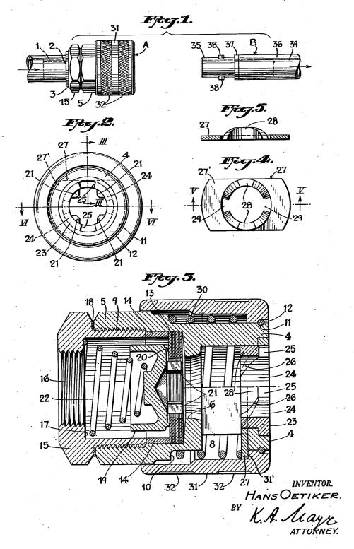
PIN-DETENT SWIVEL COUPLING WITH LOCKING MEANS
