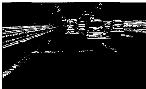
(f) BINARY HORIZONTAL EDGE IMAGE AFTER ALTERNATE PROCESSING
