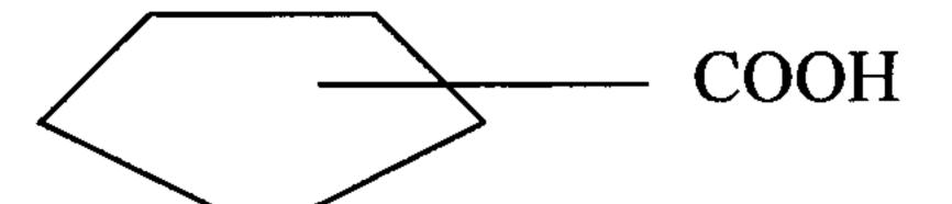
The molecular weight of naphthenic acid can extend over a large range. However, the majority of the naphthenic acid from crude oils is found in gas oil and light lubricating oil. When hydrocarbons containing such naphthenic acid contact iron-containing metals, especially at elevated temperatures, severe corrosion problems arise.
