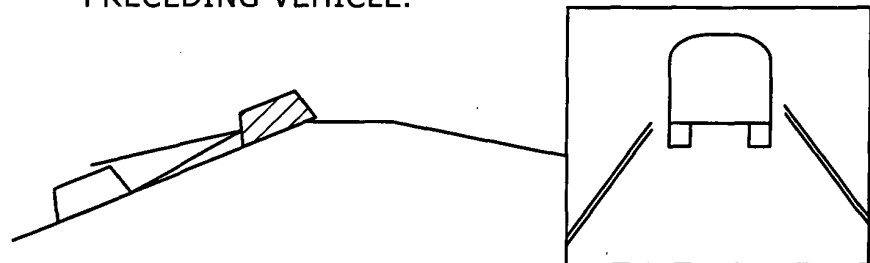
FIG. 4D SENSOR DETERMINES PRESENCE OF PRECEDING VEHICLE.
