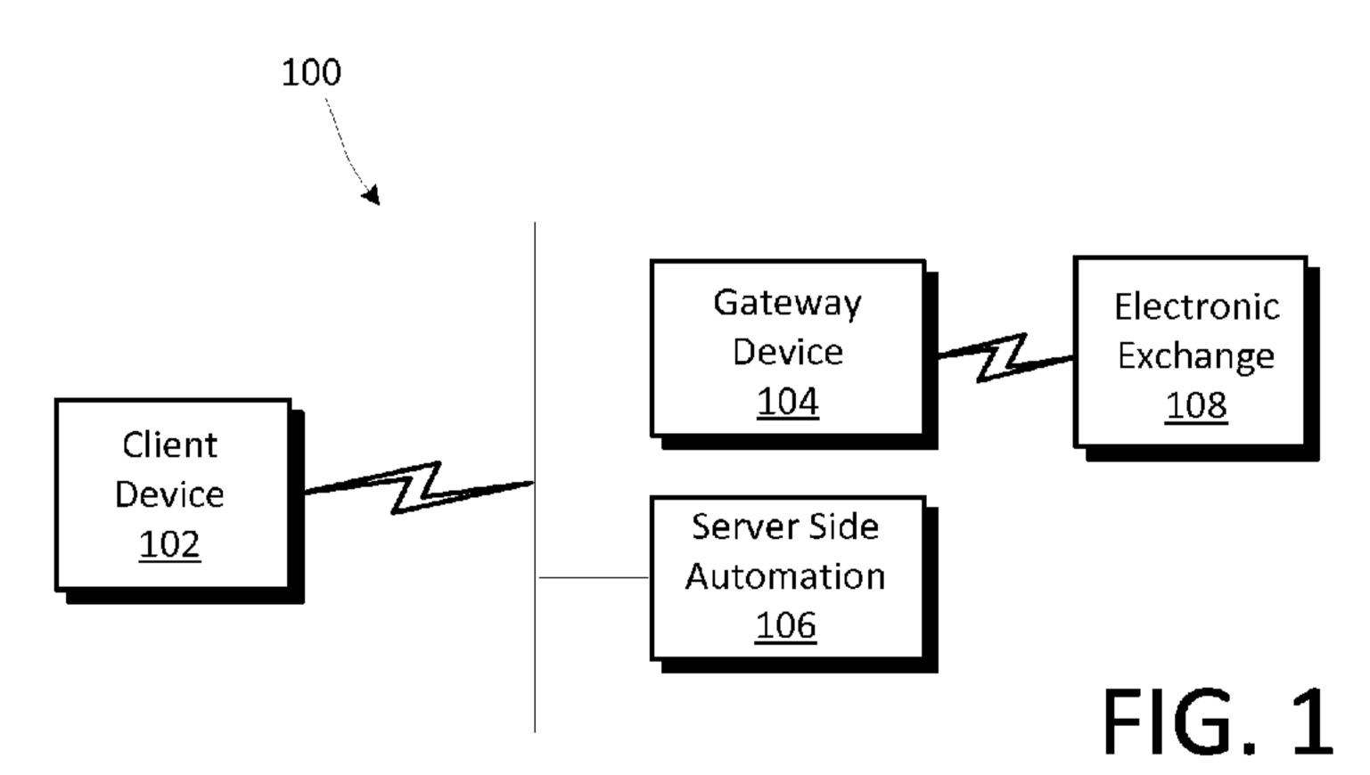
(57) Abstract: Various systems and methods for trade order processing in an electronic trading environment are provided. According to one or more embodiments, two or more trade orders are currently queued for execution at one or more electronic exchanges and are to be modified at substantially the same time. Each trade order is processed according to a priority based on each order's proximity to a particular market price, for example.
