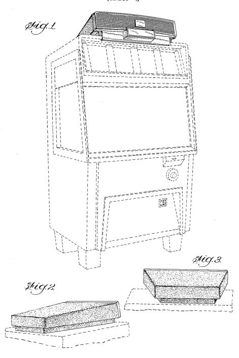
Figure 1 is a front perspective view of a phonograph cabinet showing my new design;
