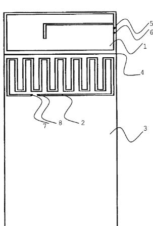
(57) Abstract: An antenna arrangement for a portable radio communication device, comprising a first (1) and a second (2) antenna element, and a conductive shield (4) connectable to a ground plane device (3), said first (1) and second (2) antenna elements are located on opposite sides of the shield (4), wherein said first (1) and second (2) antenna elements are of different types.
