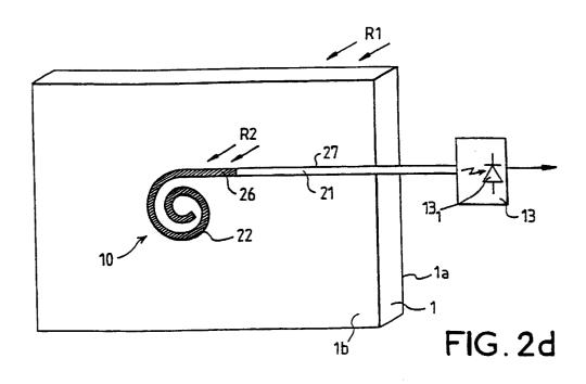
DEVICE FOR MEASURING EXPOSURE OF A SOLID-STATE IMAGE DETECTOR SUBJECTED TO IONISING RADIATION AND IMAGE DETECTOR EQUIPPED WITH SUCH A MEASURING DEVICE
