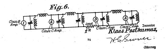
SYSTEM FOR AMPLIFYING MODULATED WAVES
