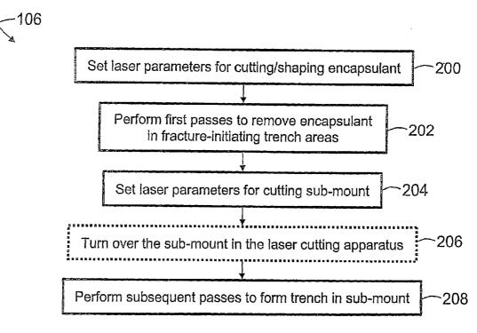
(57) Abstract: In a light emitting package fabrication process, a plurality of light emitting chips (10) are attached on a sub-mount wafer (14). The attached light emitting chips (10) are encapsulated. Fracture-initiating trenches (30, 32) are laser cut into the sub-mount wafer (14) between the attached light emitting chips (10) using a laser. The sub-mount wafer (14) is fractured along the fracture initiating trenches (30, 32).
