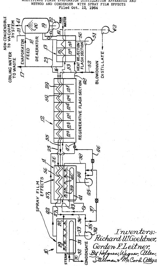
June 11, 1968 MULTISTAGE FLASH EVAPORATOR DISTILLATION APPARATUS METHOD AND CONDENSER WITH SPRAY FILM EFFECTS Filed Oct. 12, 1964 **3,388,045** APPARATUS AND
