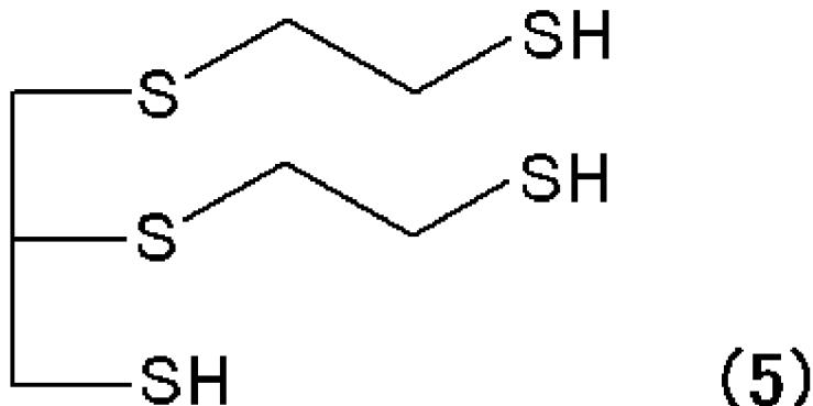
a step (a4) for adding hydrochloric acid which is a concentration of 25% to 36% to the solution containing the polythiol compound thus obtained, washing the solution at a temperature of 10°C, to 50°C to purify the polythiol compound represented by the formula (5).
