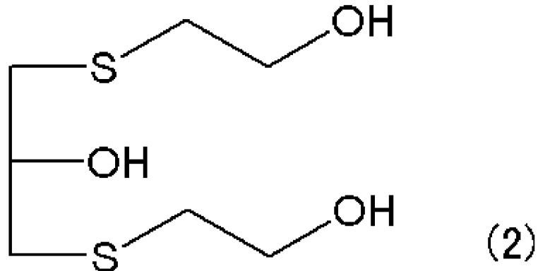
5 a step(a2) for reacting the polyalcohol compound represented by formula (2) thus obtained with thiourea in the presence of hydrogen chloride to obtain an isothiuronium salt;
