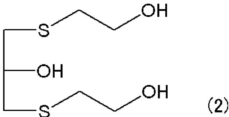
a step (a2) for reacting the polyalcohol compound represented by formula (2) thus obtained with thiourea in the presence of hydrogen chloride to obtain an isothiuronium salt;
