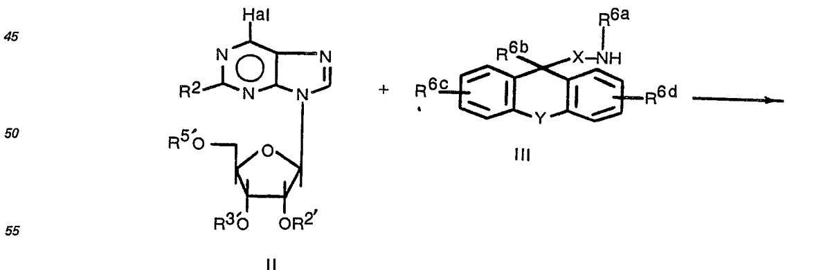
60 wherein Hal is halogen, preferably chlorine or bromine, and Y, R<sub>2</sub>, R<sub>6</sub><sup>a</sup>, R<sub>6</sub><sup>b</sup>, R<sub>6</sub><sup>c</sup>, R<sub>6</sub><sup>d</sup>, R<sub>2</sub>', R<sub>3</sub>', and R<sub>5</sub>' are as defined for formula I.
