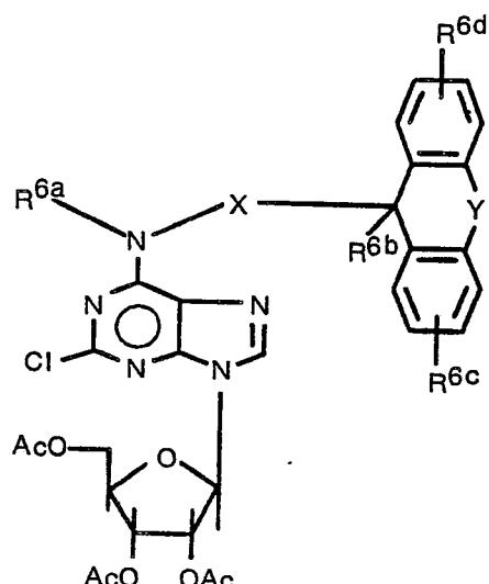
60 with R<sup>2</sup>—H, wherein Ac is acetyl; removing the acetyl groups with ammonium hydroxide, and, if desired, converting the resulting free base to a pharmaceutically acceptable acid addition salt.
