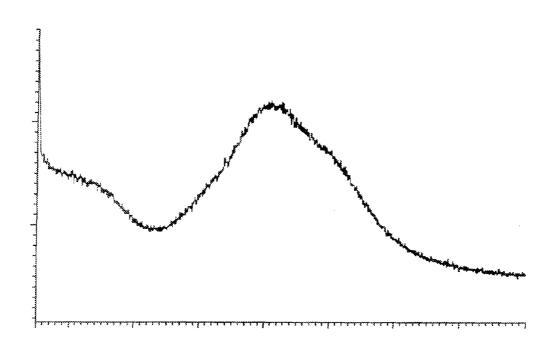
X-ray Tube: Cu(1.54060 A) Voltage: 40.0 kV Current: 40.0 mA Scan Range: 2.5000<-> 40.0000 deg Step Size: 0.0200 deg Count Time: 12.00 sec Siit DS: 1.00 deg SS 1.00 deg: RS: 0.30 mn
