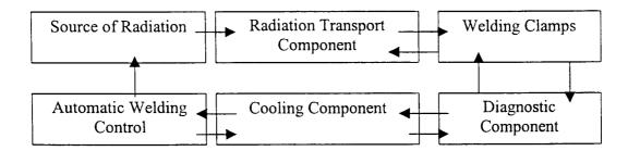
The prototype assembly consists of a set of lasers with selective radiation in the wavelength range of about 0.5 microns to about 1.3 microns. A set of lasers with re-tunable wavelength may be used instead. A unit for transportation of laser radiation is represented by a set of fiber-optics cooled with water (particularly since the required power is expected to exceed 0.53 W/cm<sup>2</sup>).
