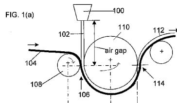
(57) Abstract: Methods for extrusion coating a substrate are provided. The methods comprise applying an extrusion coating composition to a surface of a substrate by extrusion coating. In these methods, the extrusion coating composition includes a polyolefin and an inorganic particulate material having an average particle size of no greater than 2  $\mu\text{m}$  and a particle loading of at least 20 weight percent, based on the total weight of polyolefin and the inorganic particulate material.
