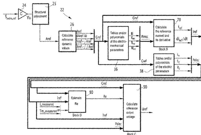
loop, from the mechanical model (36) of the loud-speaker and desired dynamic values ( $A_{ref}$ ,  $dA_{ref}/dt$ ,  $V_{ref}$ ,  $X_{ref}$ ).
