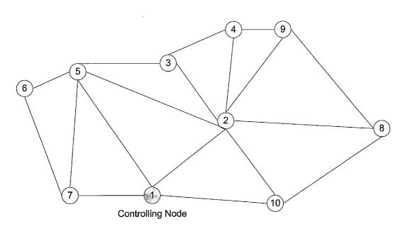
(57) Abstract: A method and a wireless communication device that implements a control node for a mesh network. Preferably, the device and method are implemented in an Access Point for an 802.11 LAN.
