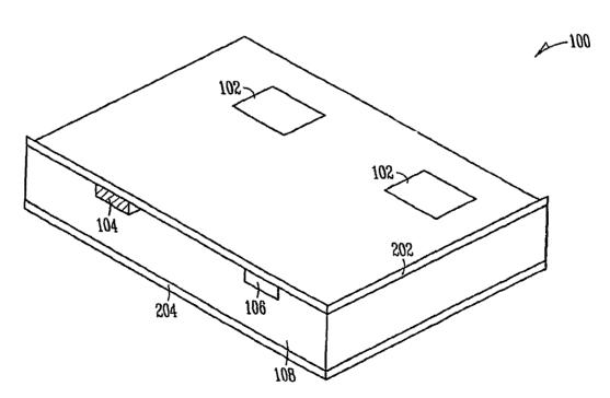
(57) Abstract: Embodiments of the invention relate to a galvanic cell comprising a first electrode, a second electrode, an electrolyte in contact with both the electrodes, a substrate adapted to support and separate the electrodes while allowing the electrolyte to move within it and contacts electrically coupled to the electrodes, wherein one or more of the electrodes comprises one or more highly reactive metals and wherein at least one of the electrodes is printed on the substrate.
