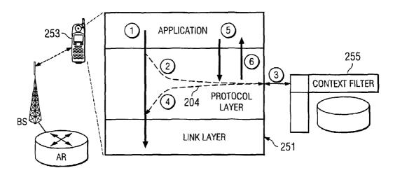
(57) Abstract: In mobile IP networks, a method of forwarding packets of a mobile node. After a mobile node moves from one cell to another which is also know as a handover, the mobile node is informed of the capability changes in the access router and the new communication path. There is also a filter mechanism (255) inside the mobile node to filter out messages that will be rejected by the new access router due to changes resulting from a handover.
