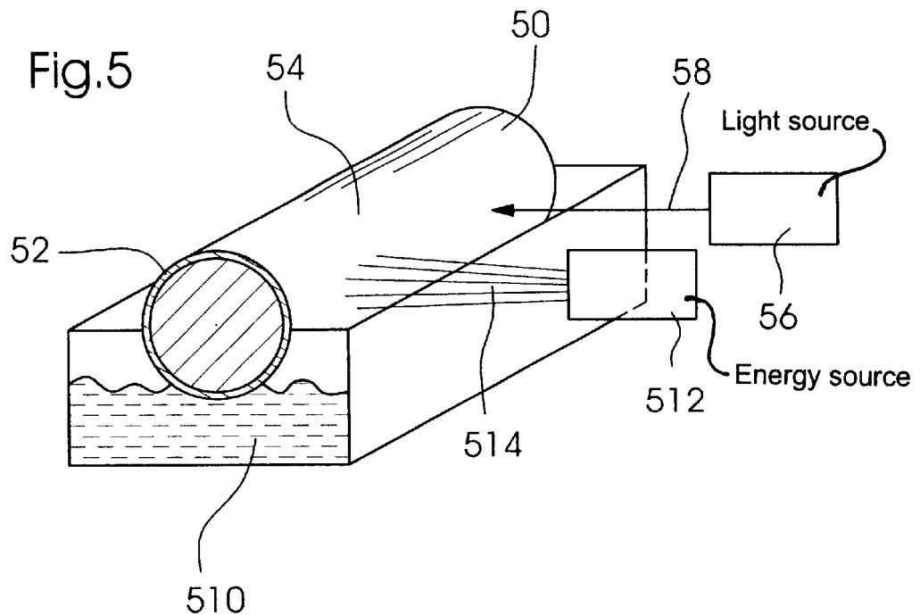
**RE-USABLE PRINTING FORM WITH A PRINTING SURFACE AND METHOD FOR FORMING IMAGES ON THE PRINTING SURFACE**
