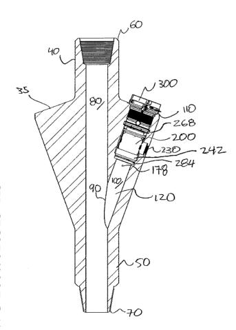
(57) Abstract: In one embodiment a method and apparatus for an improved ball dropper is disclosed. In one embodiment the method and apparatus can be used to drop various objects into the well bore from the rig. In one embodiment, when the well is pressurized the tool can be loaded with one or more items to be dropped.
