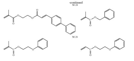
Among the structural units represented by the formula (2), the structural units derived from the compounds selected from benzyl methacrylate, phenoxy ethylacrylate and phenoxy ethylmethacrylate are preferable from the viewpoint of the dispersion stability. The water-insoluble resin of the invention has preferably one kind or two or more kinds of the structural units selected from these structural units as a hydro-<sup>25</sup> phobic structural unit (b).
