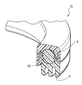
(57) Abstract: A MacPherson strut tube having an upper spring seat, a spring, a strut tube, and a ring bearing (15, 25, 35, 45, 55 and 65) disposed for engaging the spring seat, the spring and the strut tube. The ring bearing (15) comprises an upper casing (8), a lower casing (9), and a plastic ring (20) engaged between the upper and lower casings, thereby forming said ring bearing.
