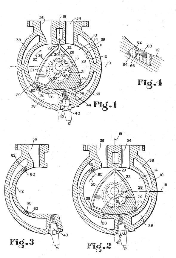
This invention relates to rotary combustion engines, and more particularly to the provision of an auxiliary ignition system for a Wankel engine.
