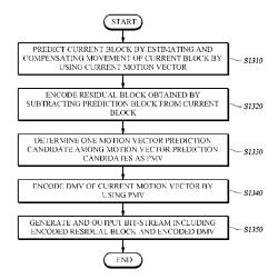
candidates from motion vectors of one or more blocks adjacent to the current block in the current frame, and means for deriving a second motion vector prediction candidate from a motion vector of the block located in the reference frame.
