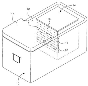
(57) Abstract: An auxiliary box placed in an insulated chamber, vessel or container to produce a controlled temperature. The auxiliary box receives a coolant, such as dry ice (CO2), and is constructed to allow controlled escape of the coolant into the chamber, vessel or container at a predetermined rate thereby controlling and maintaining the temperature ranges in the chamber, vessel or container to be cooled at a substantial constant temperature.
