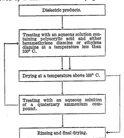
Products not conducting electricity have the property that they become electrostatically charged during further processing and during use. These electrostatic charges, which may occur by rubbing the products against each other or by rubbing the products with other bodies, give rise to various disadvantages which may show themselves in different ways dependent upon the nature of the treatment or the use.
