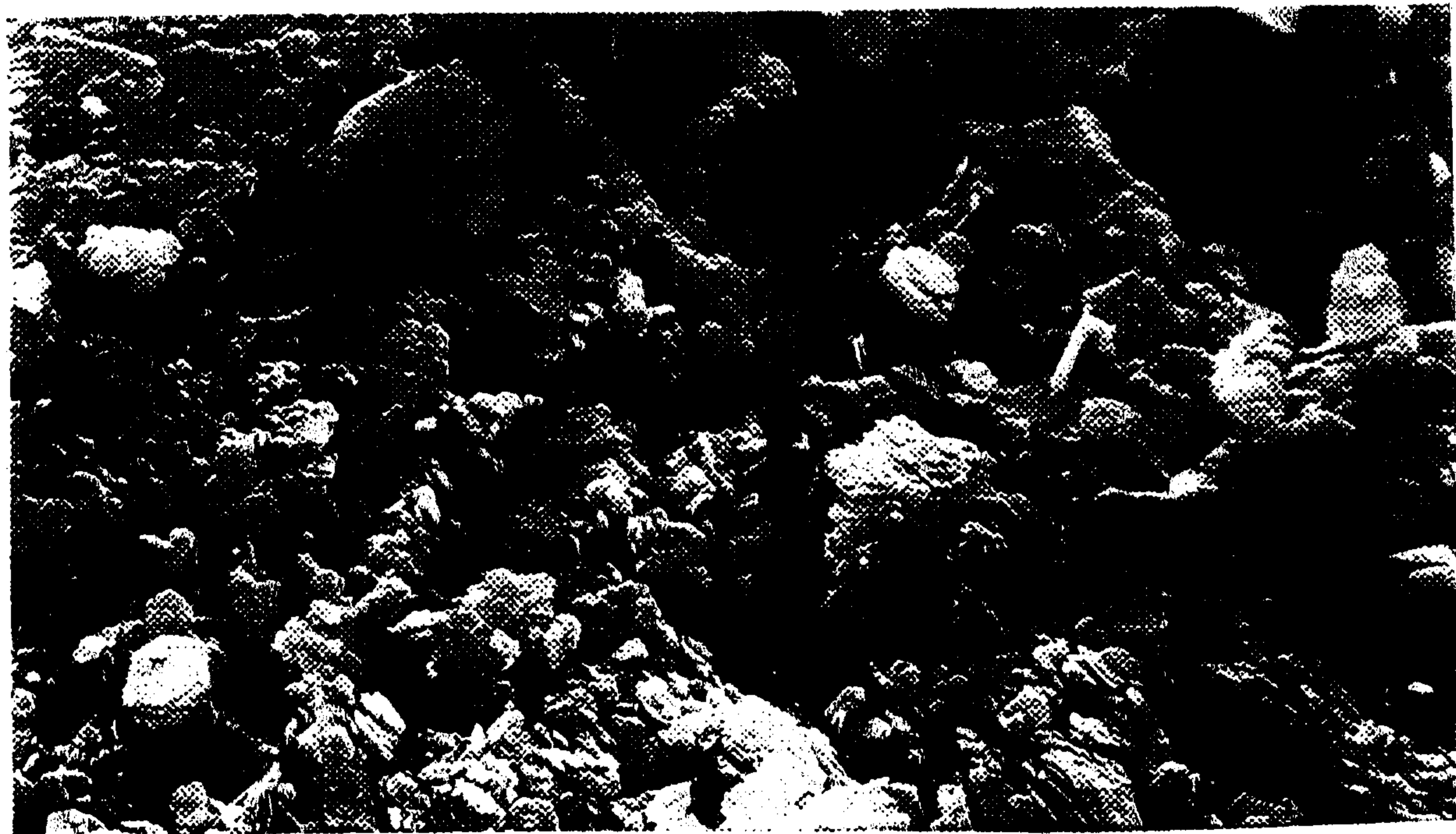
Treated Fiber, 25% Clay - 8000X
