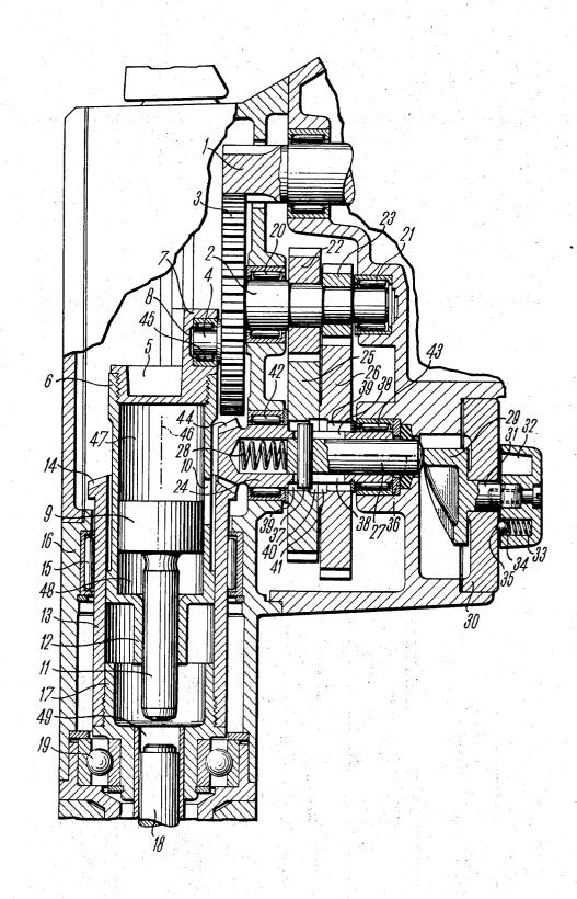
The present invention relates to a percussion or hammer drill which is operated by a motor driven gear unit which comprises first gear elements for effecting the 5 rotary movement of the drilling tool and second gear elements for reciprocating a striker in the axial direction of the tool so as to exert impacts upon the drilling tool
