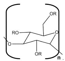
Regarding the formula of this structure, n is 10 to 4000, and each R can independently be an H or an organic group. Furthermore, the poly alpha-1,3-glucan ether compound has a degree of substitution from 0.05 to 3.0, and the compound contains two or more types of organic group. Significantly, a poly alpha-1,3-glucan ether compound herein can be an alkyl ether and/or hydroxyalkyl ether derivative of poly alpha-1,3-glucan.
