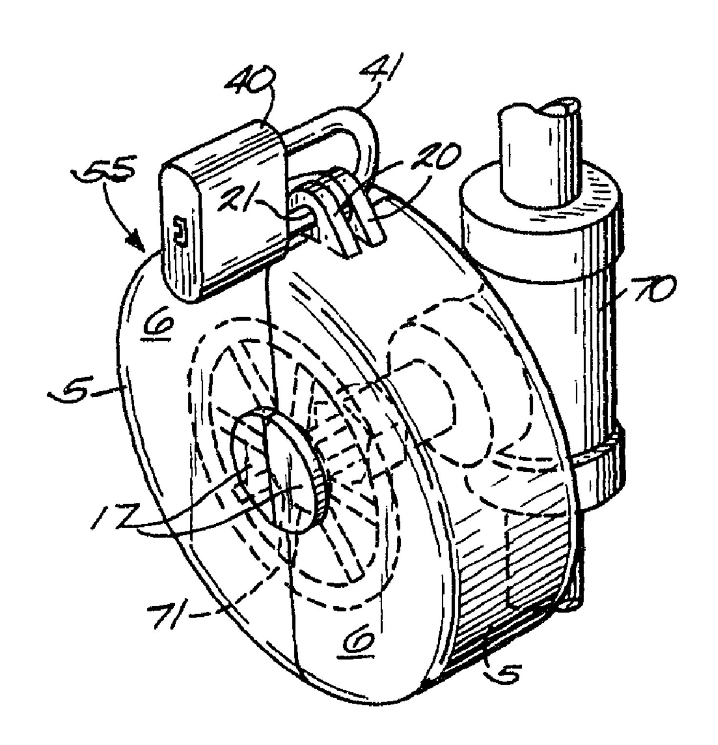
(57) An enclosure (55) for a valve handle (71) formed of two enclosure-halfs (5) of identical structure hinged together to form a clamshell enclosure for the handle of the valve.
