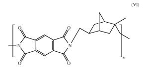
[0211] The polyimide shown in formula (VI) is typically formed from a mixture of isomeric diamines based on the mixtures (and isomers) described above. Another common polyimide of the present invention can be shown by the following formula below,
