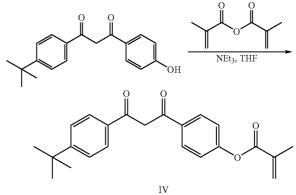
Step 5—Polymerization: An acrylic copolymer of dibenzoylmethane and mPDMS is prepared in a manner similar (AIBN initiated polymerization, precipitation addition via cold methanol) to the method for synthesizing the polymers described above, with reference to Examples 1-4.
