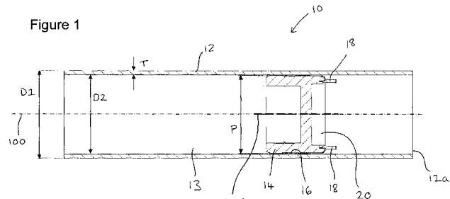
(57) Abstract: A method of sealing a plastics pipe with a plug, wherein said plug includes an electrofusion element around an outer surface thereof, said method comprising the steps of inserting said plug in a bore of the pipe and energising said electrofusion element whilst said plug and said pipe are radially urged against one another to form a seal between said plug and said pipe.
