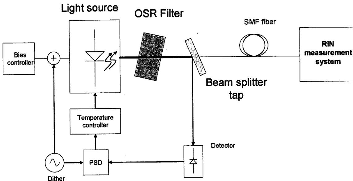
**Control loop to keep laser wavelength fixed on the filter.**
