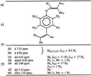
This monomer was cationically active as before, curing tack free i 10 seconds  $@100 \text{ mW/cm}^2$  @predominantly 366 nm. The resulting polymer was a flexible solid with a Tg of 85° C. (1 Hz by DMTA).
