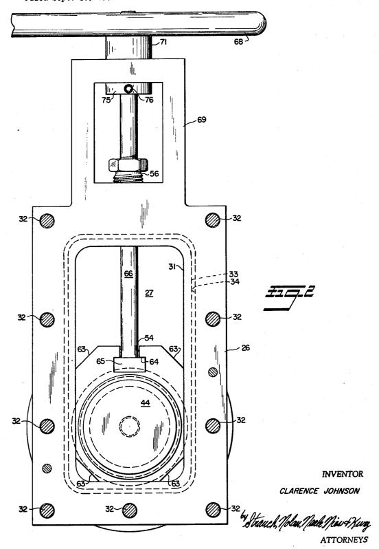
SECTIONAL BODY GATE VALVE WITH SEAT SCRAPING MEANS
